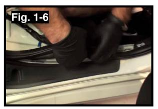
Remove the Passenger side seat belt trim panel by pulling directly towards you from the lower portion of the panel. Once lower position of the Seat Belt trim is loosened, disengage trim by sliding the panel in a downward motion. (Fig. 1-7)
