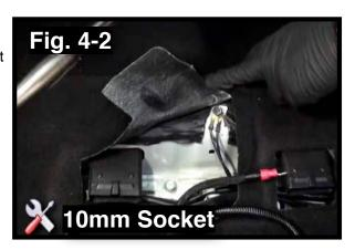
c. Install the harness ground together with the factory ground and re-install the 10mm bolt.
