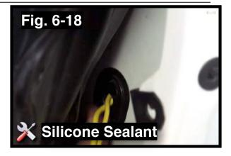
w. Using a fish pole, grab tool or modified wire coat hanger fish the power wires from the wheel well to the engine compartment.
