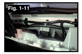
Lift the rear-seat backrest carpet locations in the cargo area exposing the channel between the rear seat and the cargo area.
