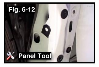
q. In the driver's side kick panel area; use a pick tool to open the inner fender harness shield.
