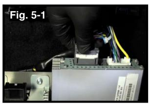
c. Plug the Black 10-pin connector from the Quick-Sync Harness into its designated receptacle on the Sub Amplifier. (Fig. 5-2)
