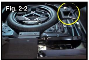
c. Run cable under the rear seat belt bolt and towards the passenger side rear threshold area.
