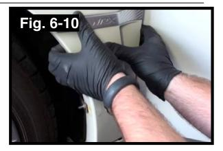
Loosen Wheel Well Liner by disengaging three (3) push in snaps. Loosening the wheel well liner will provide access to the Sun roof Drainage Cap. (Fig. 6-11)
