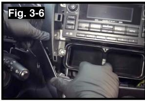
h. Once front dash bezel is loose; disconnect the climate control connectors. And remove the Front Bezel completely from the vehicle.
