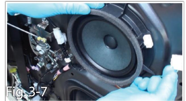
8. Remove the three 10mm bolts holding the factory speaker in place and remove speaker. (Fig. 3-8)
