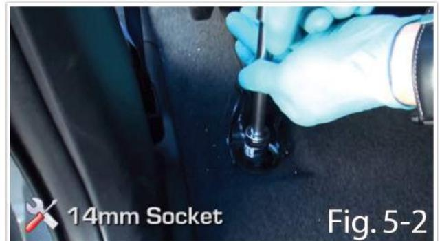
3. Slide seats to the rear and remove the two (2) front 14mm seat bolts. (Fig. 5-3)
