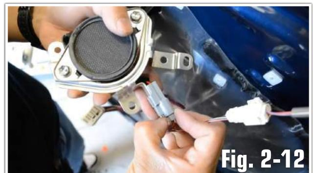
4. Position OEM Audio Plus 1" Tweeter in position and re-install dash speaker connector.
