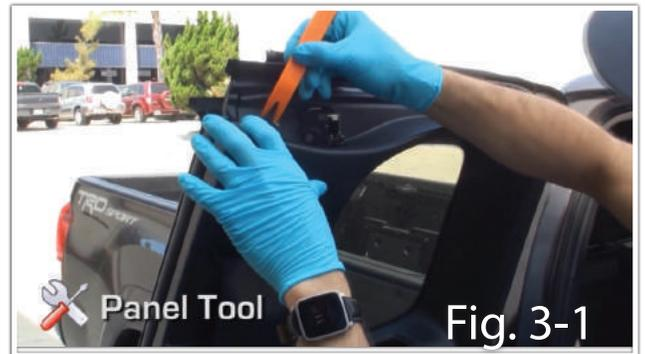
2. Use a panel or pick tool to remove the cover behind the interior door latch. (Fig. 3-2)
