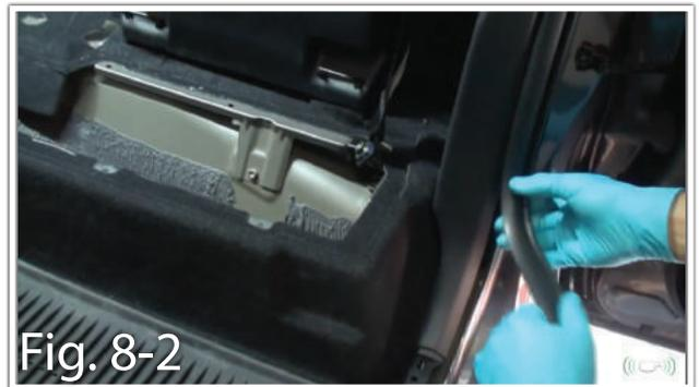
c. Apply pressure to the panel pushing towards the passenger side to disengage the locking tabs. Only the lower portion of this panel needs to be loosened to clear a pathway to run the subwoofer umbilical through the cavity where the under seat storage panel installs. (Fig. 8-3)
