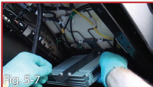
5. Use the provided 10mm bolts to secure the amplifier bracket assembly to the underseat frame. (Fig. 5-8)
