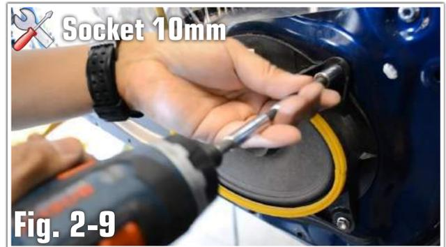
3. Mount the 6x9 OEM Audio Plus speaker by using the four 10mm bolts and re-install 6x9 speaker connector.
