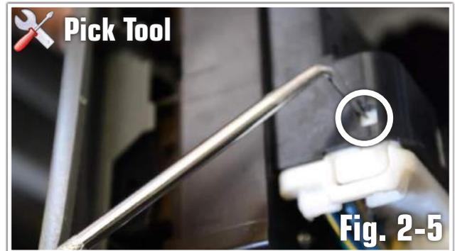
5. Use a pick tool to remove the cover behind the interior door latch. **(Fig. 2-6)**
