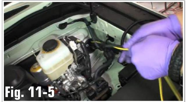
g. Run power wires to the battery by following the direction of the factory wiring harness towards the battery. Secure using cable ties as necessary. **(Fig. 11-6)**
