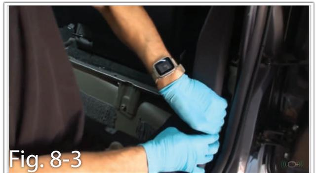
d. Run the length of the subwoofer umbilical alongside the driver's side threshold and through the available path to this area. (Fig. 8-4)
