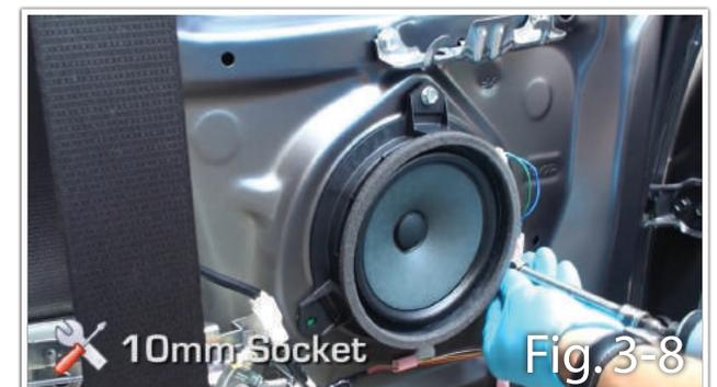
10. Reinstall door in reverse order taking time to ensure all clips are engaged. Failure to securely reinstall door panel may result in rattles.
