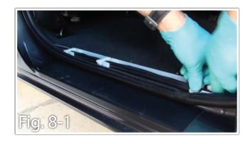
b. Remove the weather stripping on the driver side to access the side rear panel (Fig. 8-2)
