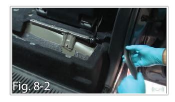
c. Apply pressure to the panel pushing towards the passenger side to disengage the locking tabs. Only the lower portion of this panel needs to be loosened to clear a pathway to run the subwoofer umbilical through the cavity where the under seat storage panel installs. (Fig. 8-3)
