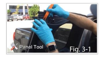
2. Use a panel or pick tool to remove the cover behind the interior door latch. (Fig. 3-2)
