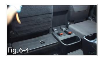
e. Remove the front and rear center console mats. Remove the four 10mm bolts. Remove the driver's side and passenger side rear seat belt assemblies. (Fig. 6-5)
