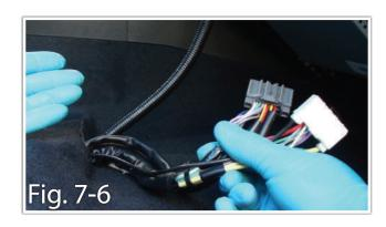
g. Plug the White and Gray 22-pin connectors from the Quick-Sync Harness into their designated receptacles on the DSP Amplifier. The white connector inserts into the receptacle towards the rear of the vehicle. Note: You want to make sure the Quick-Sync Wiring Harness has enough slack so that the cable is in a rested position even when the driver's seat is pushed all the way back. (Fig. 7-7)
