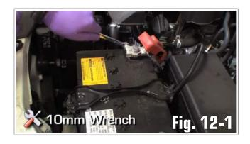
b. Install the ring terminal of the fuse holder lead.(Fig. 12-2)
