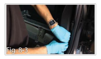
d. Run the length of the subwoofer umbilical alongside the driver's side threshold and through the available path to this area. (Fig. 8-4)
