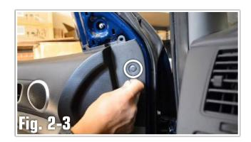
3. Use a panel tool to remove the window/door lock control panel. **Note**: Insert tool between the front edge of the panel of the trim to remove.
