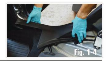
g. Remove the front Passenger side threshold panel by pulling straight up to remove. **(Fig. 1-5)**
