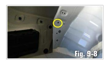
i. Install the Mounting Bracket using provided wing nut and 13mm socket or wrench to tighten. Note:
