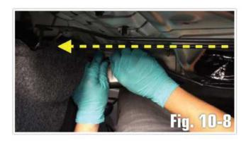
k. Continue to run the Power Wire along the factory channels towards the drivers side kick panel
