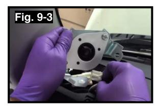
d. Mount the OEM Audio Plus dash speaker by using the two 10mm bolts. (Fig. 9-4)
