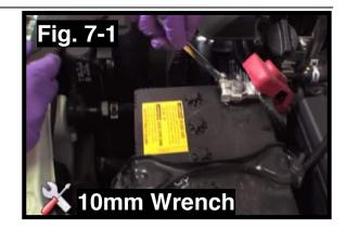
Install the ring terminal of the fuse holder lead then re-install the 10mm bolt and tighten. Note: Do not install fuses at this time. (Fig. 7-2)
