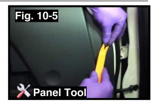
g. Use panel tool to disengage the clips behind the door panel one at a time. Start at the bottom, then the sides and finish at the top. Use gentle force to remove door panel. (Fig. 10-6)
