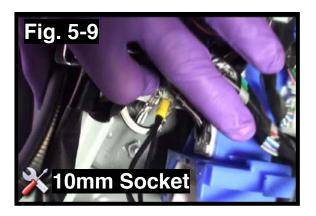
j. Reinstall the factory speaker module using a 10mm socket wrench. (Fig. 5-10)
