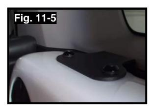
f. Install the two provided 10mm bolts into the bottom subwoofer mounting bracket. Tighten lower bracket completely. Tighten top bracket mounting hardware completely.
