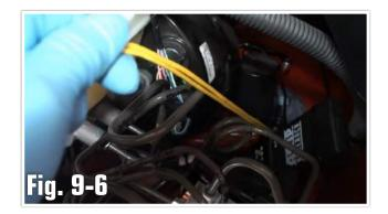
h. Secure any wire slack to existing factory wiring.Use cable ties as necessary.
