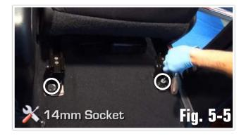
g. Slide seats to the rear and remove the two (2) front 14mm seat bolts. **(Fig. 5-6)**
