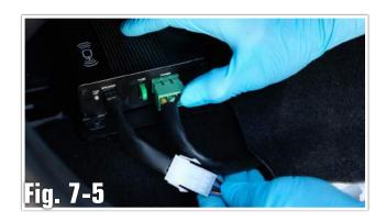
c. Plug in the provided **Factory Amplifier Bypass Connectors** to the factory 10-pin and 12-pin connectors. (Fig. 7-6)
