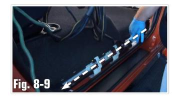
k. Continue to route umbilicals along side the rear of vehicle behind the rear insulation padding towards the drivers side of the vehicle (where the subwoofer will mount). (Fig. 8-10)
