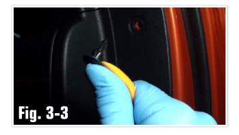
4. Use a panel tool to remove the cover behind the interior door latch. (Fig. 3-4)
