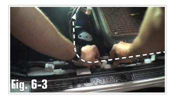
5. Run the cable under the carpet and exit under the seat through the center opening pull about 3-4 inches of slack. **(Fig. 6-4)**
