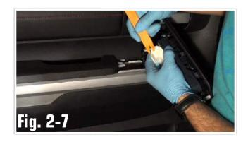
9. Use gentle force to remove door panel. Start at the bottom, then the sides, and finish at the top. (Fig. 2-8)
