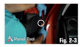
3. Use a panel tool to remove the cover behind the interior door latch and remove the #2 Phillips screw. (Fig. 2-4)
