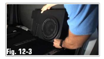
c. Install the three (3) provided 10mm bolts into the subwoofer mounting arms. Tighten by hand initially.If binding occurs remove the bolt and repeat steps.
