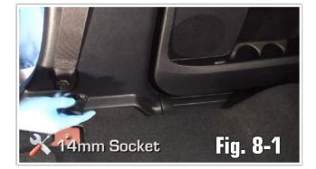
b. Remove the passenger side rear threshold. (Fig. 8-2)
