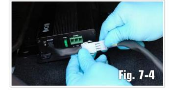
4. Connect Power & Ground (GreenConnector) to the designated Greenreceptacle on the SUB Amplifier. (Fig. 7.5)
