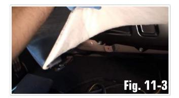
c. On the drivers side lift the padding - identify the drivers side rear mounting location and return the padding to it's original position.
