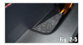
5. Use a panel tool to remove the window/door lock control panel. Note: Insert tool between the front edge of the panel of the trim to remove.
