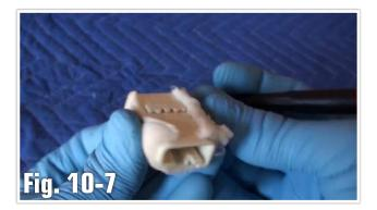
4. With the wire you intend on removing in your grasp, use a precision tool to disengage the locking tab within the connector housing securing the terminal. (Fig. 10-8)
