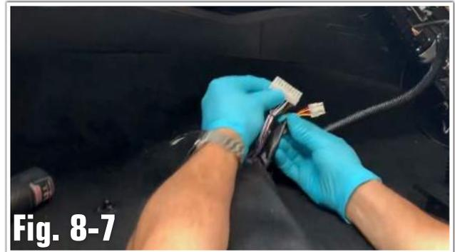
h. Plug the remote cable and 20-pin from the Quick-Sync Harness into their designated receptacles on the DSP Amplifier. The 20-p connector inserts into the receptacle towards the front of the vehicle.
