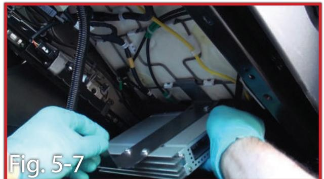
5. Use the provided 10mm bolts to secure the amplifier bracket assembly to the underseat frame. (Fig. 5-8)
