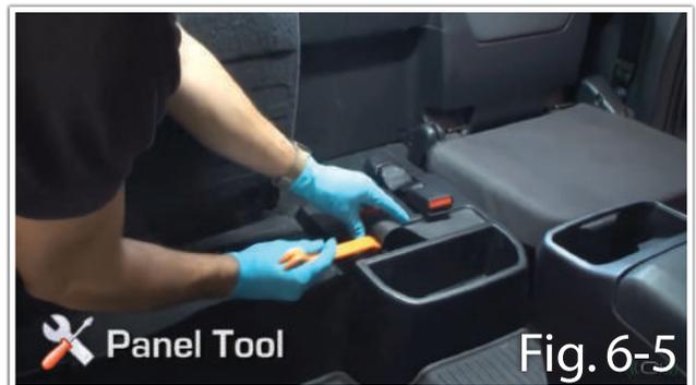
f. Release the lock and fasten the floorboard to the seat bottom. Disengage the two guides and remove the lower console box. (Fig. 6-6)
