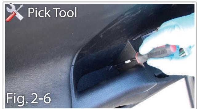
6. Remove #2 Phillips screw behind the door latch.
