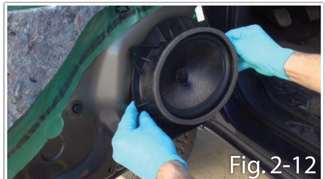
4. Reassemble the door in reverse order, taking time to ensure all clips are engaged.
