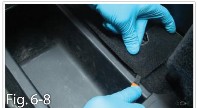
i. Remove under seat storage panel. Disengage floorboard. Using a plastic panel tool remove the twelve pushing snaps securing the under seat storage panel in place. (Fig. 6-9)
