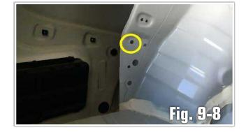
i. Install the Mounting Bracket using provided wing nut and 13mm socket or wrench to tighten. Note:
