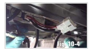
f. Postition the O+Amplifier Assembly and Wiring Harness as seen below prior to mounting:
