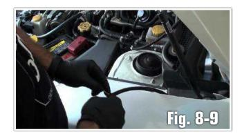
I. Run the loomed power wires from the wheel well to the battery following the factory wiring. Secure using cable ties as necessary. **(Fig. 8-10)**
