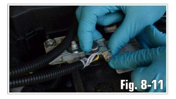
o. Connect the power wires to the fuse holder using the pre-installed crimp-solder-seal butt connectors. These special connectors have built in solder and heat shrink. Use wire stripper and strip 3/8" off the end of each power wire. **(Fig. 8-12)**
