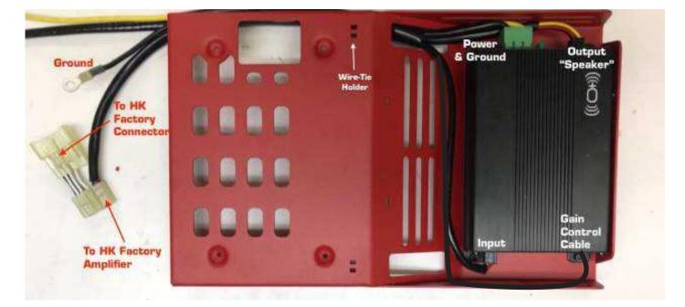
g. Install O+ Amplifier Bracket (and Harness) using
