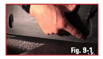
b. Disengage the six (6) clips holding the driver side trunk liner into position. Remove by prying the top cap of the clip and removing the insert of the side trunk liner clips. **(Fig. 9-2)**
