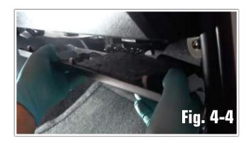
i. Run Passenger side of Quick-Sync Wiring Harness entering the channel along the side of the glovebox to above the glovebox assembly. **(Fig. 4-5)**
