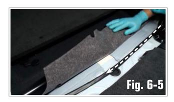
i. Run cable under the Driver side rear side panel to the far rear cargo area.
