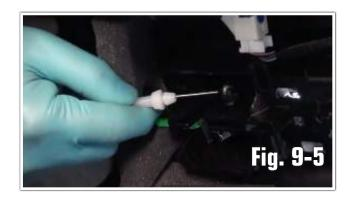
f. Disconnect window/door lock control connectors from the panel. Use of a pick tool or precision screwdriver is needed to release connector.
