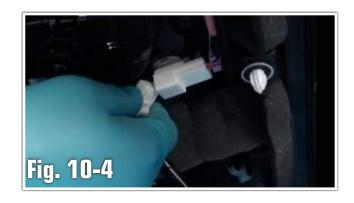
e. Remove the three (3) 10mm bolts holding the factory 6.5" factory speaker in place, disconnect the connector, and remove speaker. (Fig. 10-5)
