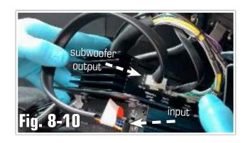
2. Connect the Subwoofer Umbilical (CO9) with the SPU-Output Connector (C13), to the SPEAKER receptical on the SUB Amplifier.
