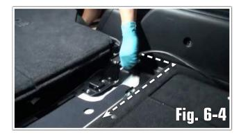
h. Run cable from passenger to driver side under the carpet along the channel between the rear seat and the cargo area. (Fig. 6-5)
