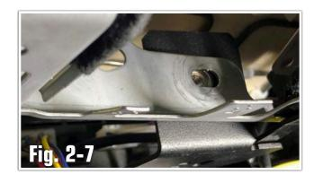
i. Use the provided 10mm bolt to secure the amplifier bracket assembly to the under-seat frame.
