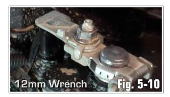
m. Install the ring terminal of the fuse holder lead.
