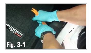
b. Remove the Passenger side kick panel by unscrewing the black locking tab (counter-clockwise) and gently pulling the panel away.
