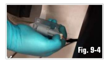
e. Remove door latch assembly from the door panel by unsnapping and lifting the door latch connectors. Note: Connectors need to be reassembled in the same orientation — white on top, green on bottom.
