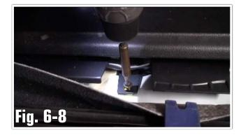
k. Using a pick tool remove the trim panel of the floor cargo net hook exposing the 10mm bolt. Remove the 10mm bolt and hook assembly. (Fig. 6-9)
