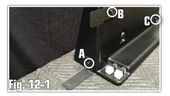
2. Place the three subwoofer brackets onto the subwoofer and attach using the three 10mm bolts. bracket A mounts to the side of the enclosure, and brackets B and C on the rear.
