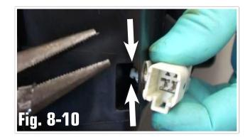
With the factory connector loose from the enclosure, take note of the wire orientation. The green wire is positive and the black wires are negative. Use a marker to note the placement, if helpful. The empty slots of this connector will remian empty. **(Fig. 8-11)**
