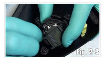
3. Install the OEM Audio Plus tweeter in the same orientation as the factory tweeter by aligning it with the locking tabs.
