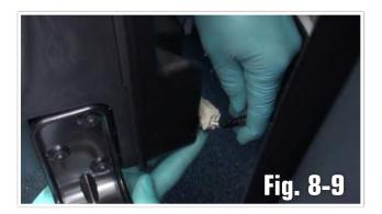
Using Needle Nose Plyers remover the factory male sub connector by compressing the white locking release found in the cavity of the factory sub enclosure.
