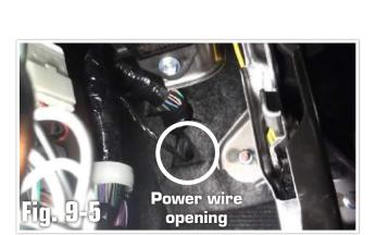
g. Once enough slack is visible, pull the full length of the power wire through under the hood (Fig. 9-6).You want just enough length to reach your battery.Cut any additional slack. Note: Avoid interference with accelerator and brake pedals.
