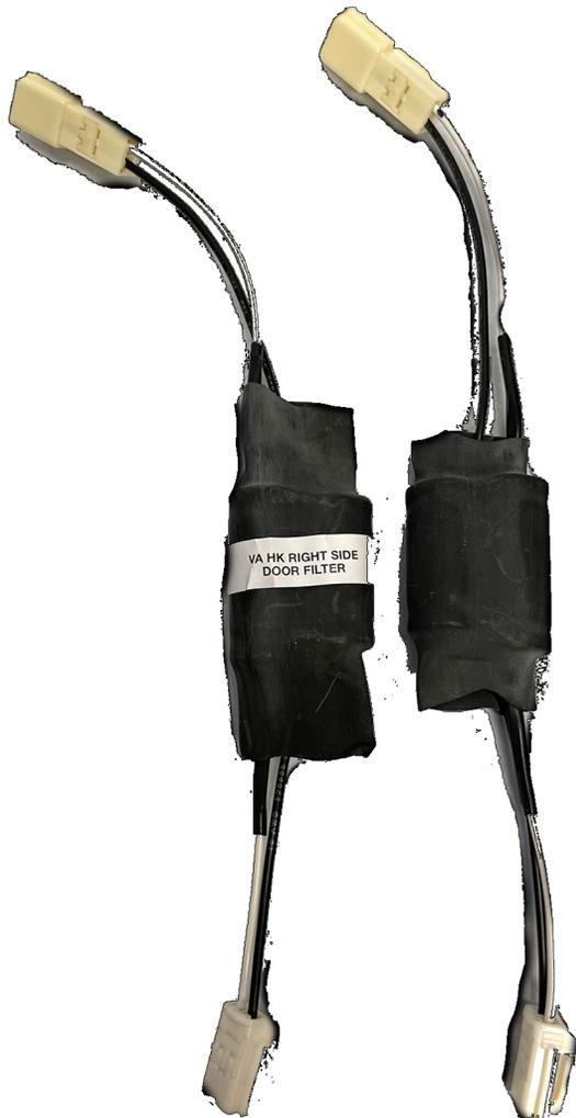
***Acoustic Correction Filters*** install in-line in front doors **between** the factory connector and factory Speaker. The below QR Code will take you to the door removal process (use your phone camera):
