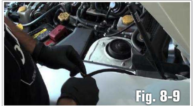
l. Run the loomed power wires from the wheel well to the battery following the factory wiring. Secure using cable ties as necessary. **(Fig. 8-10)**
