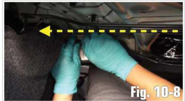
k. Continue to run the Power Wire along the factory channels towards the drivers side kick panel
