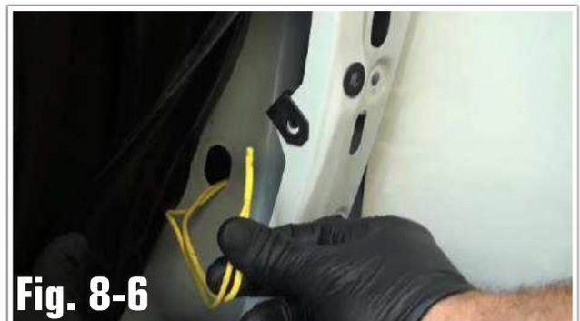
h. Once the power wire installation is completed under the dash area, secure any wire slack to existing factory wiring. Use cable ties as necessary. Reinstall Drivers side Kick Panel and threshold.
