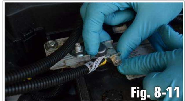
o. Connect the power wires to the fuse holder using the pre-installed crimp-solder-seal butt connectors. These special connectors have built in solder and heat shrink. Use wire stripper and strip 3/8" off the end of each power wire. **(Fig. 8-12)**
